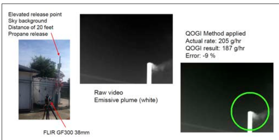
Figure 10: QOGI detection for a hydrocarbon plume released from a stack.
