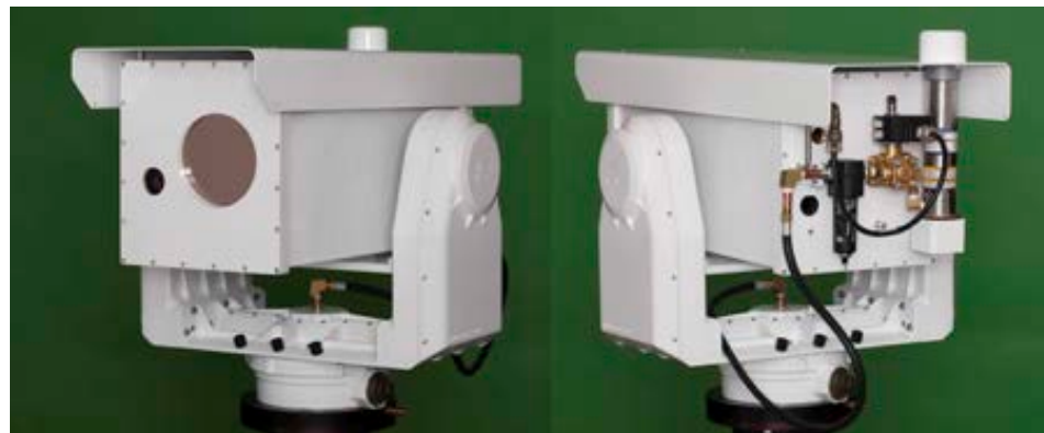
354 Figure 14: Rugged enclosure for IR optical gas imager
