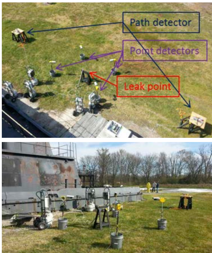
Figure 17: Field testing to compare IntelliRed™ system to point and path hydrocarbon detectors.
